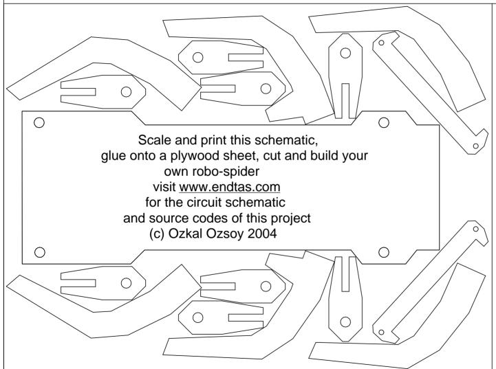
middle legs (2 total) will move up-down only, while the front and aft legs (4 total) will move forward-reverse.
