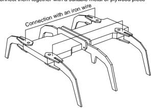
Finished spider assembly ready for the circuits' montage
